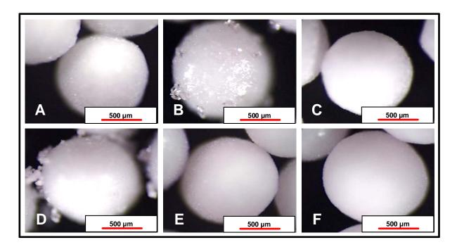
Fig. 4. O pticals tereo-photomicrograph s of particles coated with Eudragit E PO (A), Shellac (B), AQOA T (C), Matrix 1 (D), Matrix 2 (E) and Matrix 3 (F).
