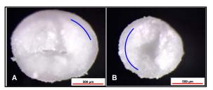
Fig. 3. Stereo-micrographs cross-section of coated particles with Matrix 3(A) and Matrix 2(B).
