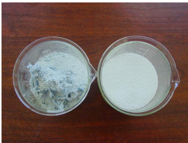
Fig. 7. Pictures of coating particles without (left) and with (right) using automatic control process (Experiment B: Q_r = 100 \text{ m}^3 \cdot \text{h}^{-1} , P_p = 1 \text{ bar} , Q_s = 18 \text{ g} \cdot \text{min}^{-1} ).
