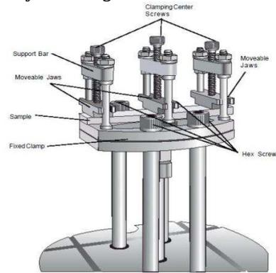
Figure 3. Clamp assembly of DMAQ800
