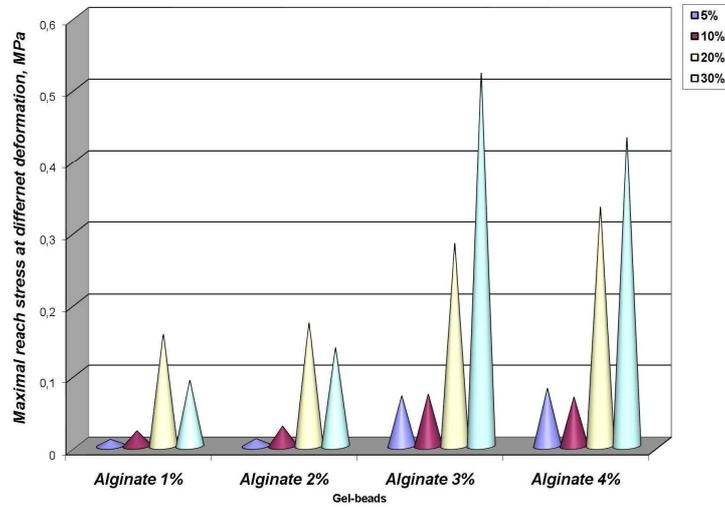
Figure 10. Necessary stress for reaching the set deformation for immobilized preparation.
