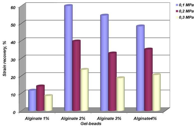
Figure 9. Relaxation degree for different Ca-alginate beads.
