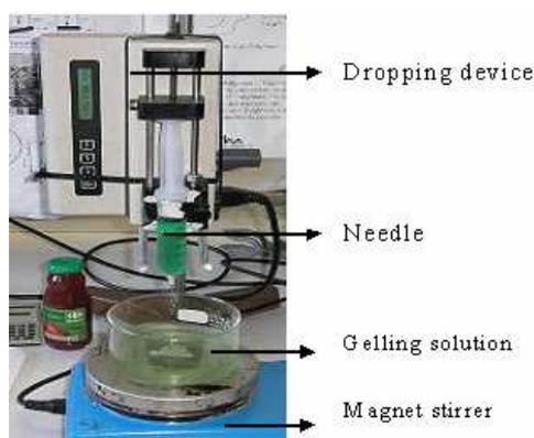
Figure 1. Device for immobilized cell preparation.
