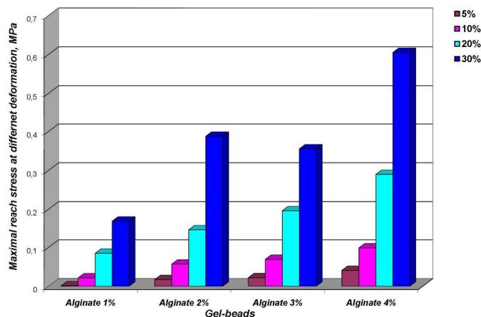
Figure 7. Necessary stress for reaching the set deformation
