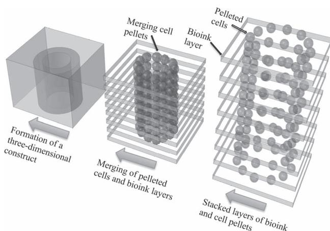
**Figure 3.** Schematic illustration of the bio-printing and self-assembly process taking form for the generation of a three-dimensional construct coupled with bioreactor time.
