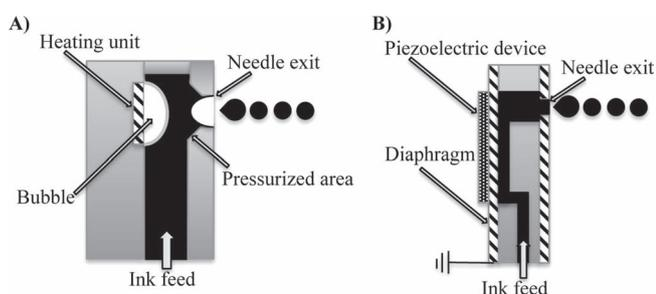
**Figure 1.** Schematic representations: A) thermal and B) piezoelectric ink-jet printing system.<sup>[7]</sup> Note that through both systems in practise the generated droplets are twice the diameter of the inner bore diameter of the explored needle. It is also noteworthy to bear in mind that both these systems apply their driving forces directly on the media, which is detrimental when handling sensitive advanced materials such as living cells.
