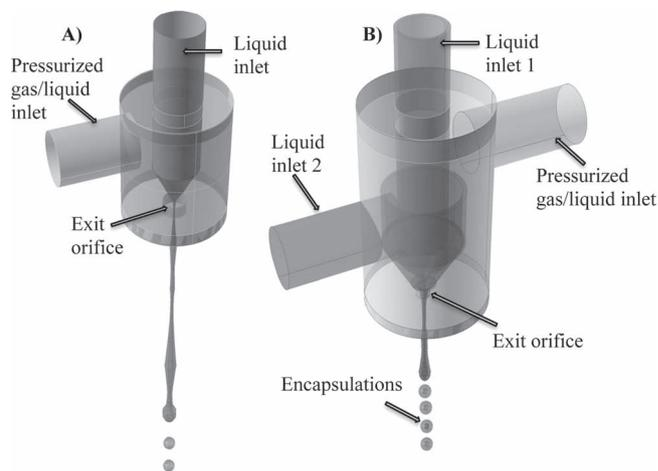
**Figure 4.** Schematic depictions: A) a single and B) a coaxial or concentric needle AABJ device. Note that driving forces are applied indirectly on the media over the exit orifice, thus being harmless when handling living cells and embryos.
