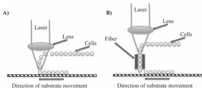
**Figure 2.** A) Characteristic schematic diagram depicting the fed cells being grabbed by the laser and subsequently being placed on a substrate. B) The scheme illustrates the fed cells being guided through a fibre for placement on a substrate.<sup>[9]</sup>
