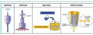
Figure 3. (Capsulae  $^{\otimes}$  ): Schematic representation of the main encapsulations systems used in the food industry.
