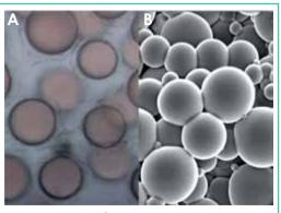
Figure 4. (Capsulae<sup>®</sup>): Microcapsules produced using emulsion-based techniques (A: coacervation; B: interfacial polymerization).
