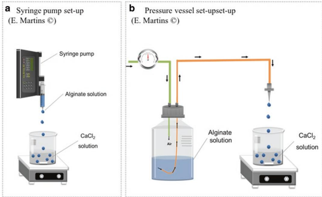
**Fig. 3** Assembling for extrusion/dripping production of alginate beads
