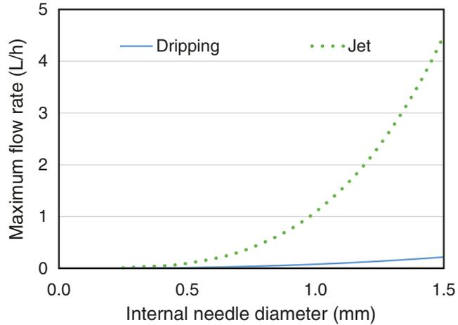
**Fig. 2** Influence of the droplet diameter on the maximum productivity
