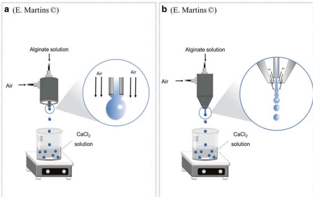
**Fig. 9** Assembling for alginate bead production using coaxial air flow
