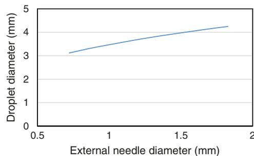
**Fig. 5** Size of the droplet,  $d_p$ , versus the external needle diameter,  $d_e$  (surface tension of the extruded solution 73 mN/m at 20 °C)
