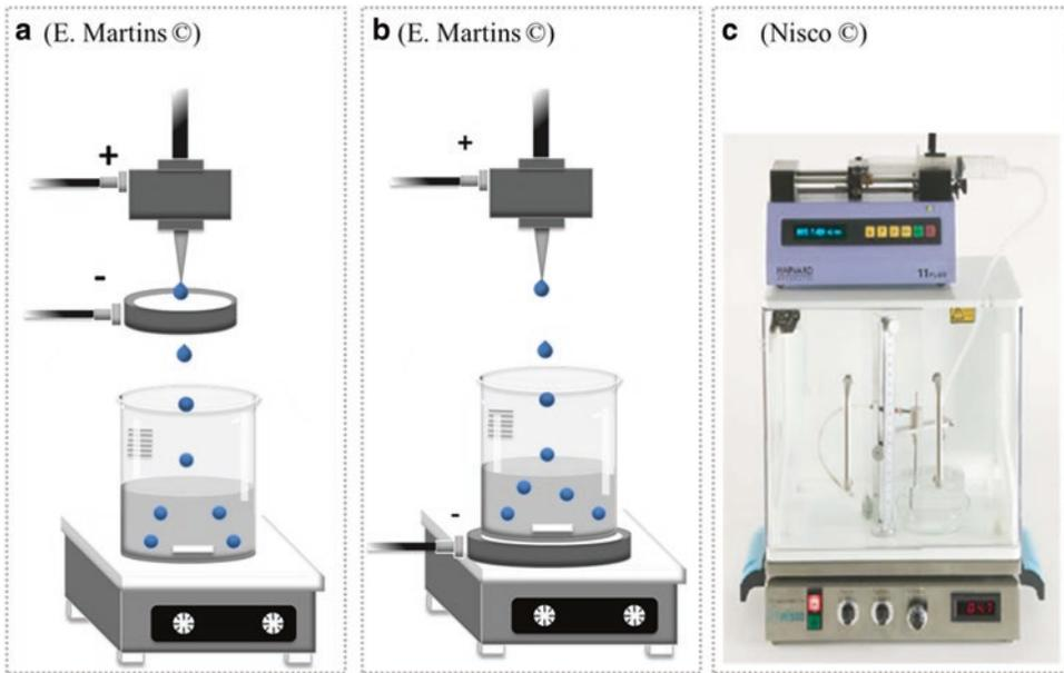
**Fig. 8** Assembling for production of alginate beads by electro-dripping
