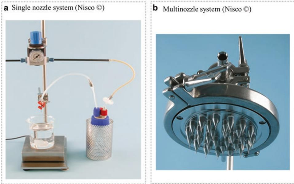
**Fig. 6** Assembling for dripping under dropwise and simple gravity regime
