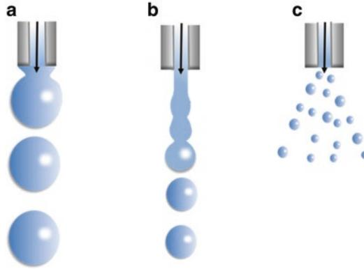
**Fig. 1** Dripping regimes: (a) Dropwise, (b) Jet-breaking, (c) Spray regime (E. Martins ©)
