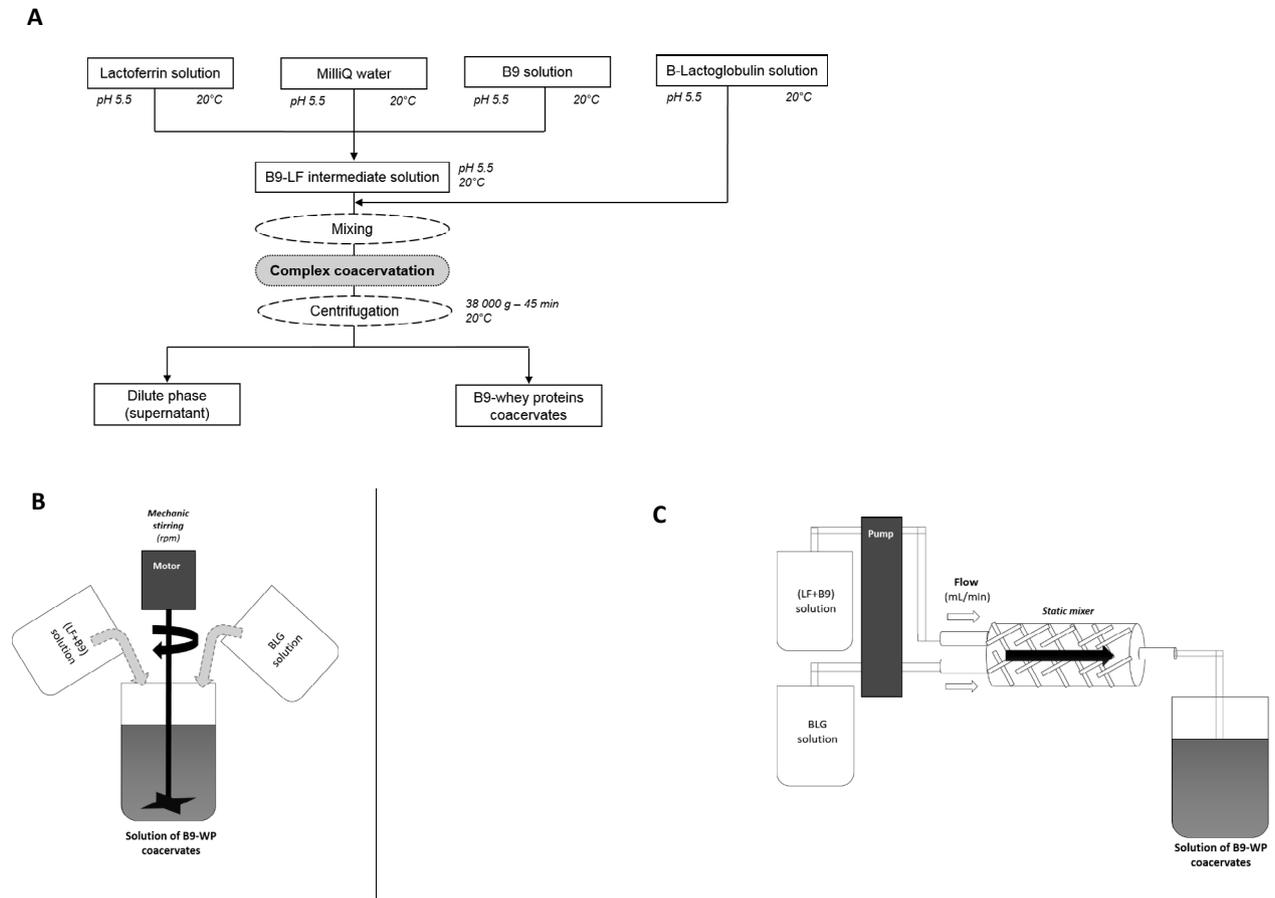
**Fig. 1.** Schematic diagram for the of production of B9-WP coacervates (A) and the device used for batch mixing by mechanic stirring (B) or continuous mixing by static stirring (C).
