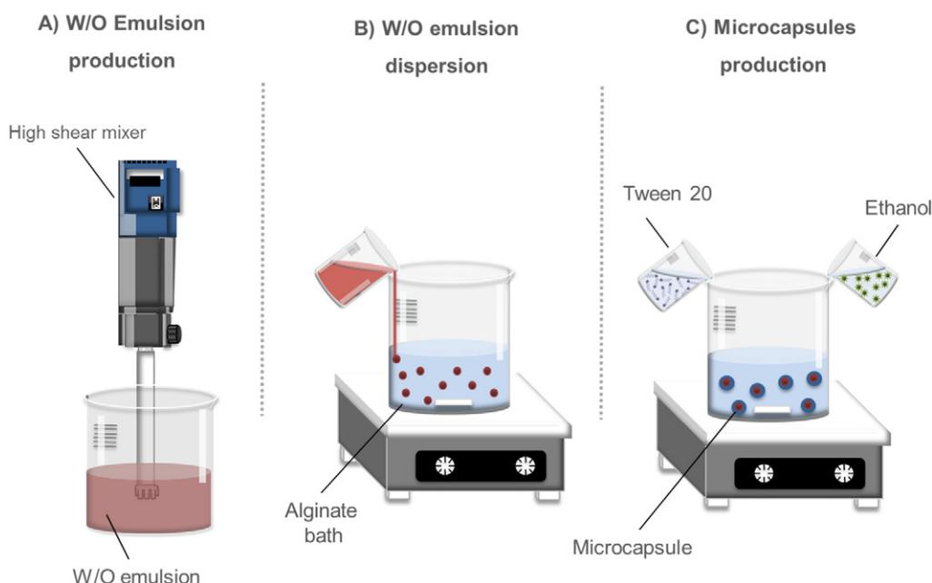
Fig. 1. Schematic representation of the experimental set-up used to produce microcapsules by inverse gelation using W/O emulsions.
