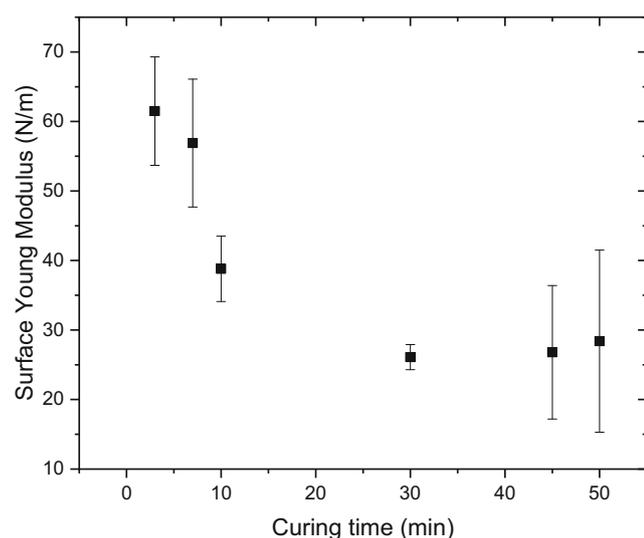
**Fig. 7** Surface Young modulus (N/m) of wet capsules as function of curing time. At the 0.05 level, the populations means were significantly different
