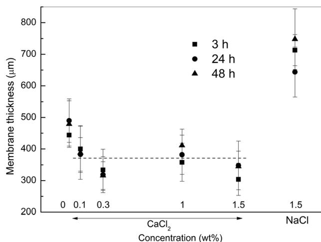
**Fig. 9** Evolution of the membrane thickness after different storage times in distilled water,  $\text{CaCl}_2$  or  $\text{NaCl}$  solutions. Curing time in alginate solution = 30 min. At the 0.05 level, the populations means were significantly different
